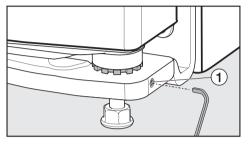
■ Unscrew threaded pin ① by a maximum of one turn using the allen key supplied.
